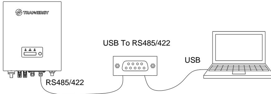
Figure 6-2 RS-485/422 Communication Diagram
